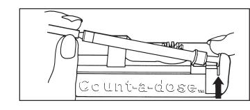
**4.** Place the plunger against the flat side of the raised area as shown above. The flanges will seat in their notches properly only if they are lying horizontally. Slip the barrel of the syringe under the clip into the channel as shown below.
