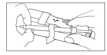
**10.** Return the **bracket** to zero by moving the dial back to the **minus sign** (-). The bracket is very flexible and could be dislodged or bent if returned by pushing with the palm of your hand.
