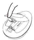
2. Remove the old battery and replace with two 1.5V AAA alkaline batteries.
